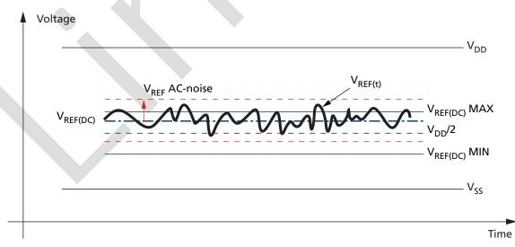
The voltage levels for setup and hold time measurements are dependent on  $V_{REF}$ .  $V_{REF}$  is understood as  $V_{REF(DC)}$ , as defined in the above figure. This clarifies that DC-variations of  $V_{REF}$  affect the absolute
